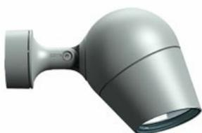
spotlight rotation symmetrical 80° (± 40°), wide beam, LED, 1600 lm, 3000 K, CRI > 80, electronic converter, Total power: 24 W
